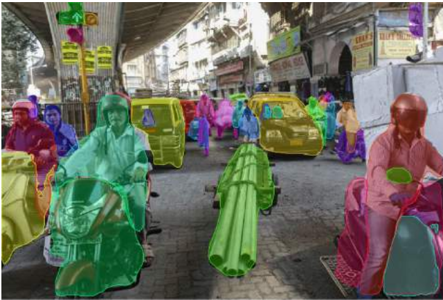
Figure 4: Efficient representations of road-agents in dense traffic. Instance segmentation helps reduce occlusions by reducing background clutter otherwise present in typical bounding box representations. These representations are used in our tracking by detection algorithm. The different colors simply denote individual road-agents.
